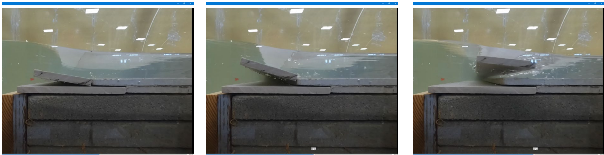
Figure 9: Failure sequence for uplift of crest cap upstream from a longitudinal crack. Elapsed time is less than 1 second.
