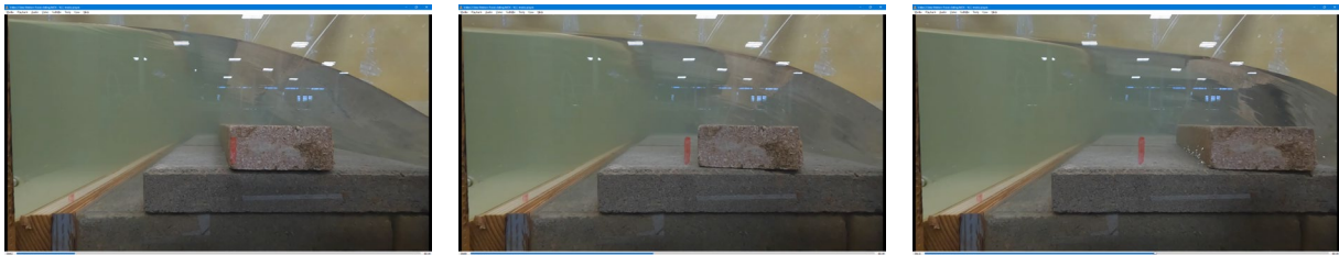
Figure 7: Sliding failure of a 40-mm (1.57-inch) concrete paver block. Flow is left to right, and time increases from left to right. Elapsed time from the first image to the last is about 1 second.
