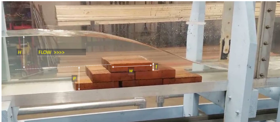
Figure 4: Initial flume testing, with illustration of key variables.
