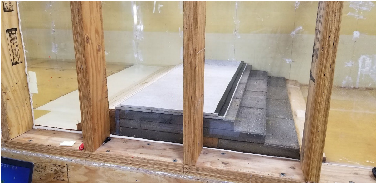
Figure 8: Dam and crest cap configuration for a sealed-downstream-edge test.
