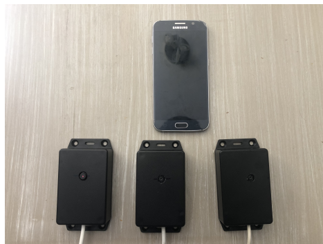
Figure 4.9. Android device and the three camera node sensors.
