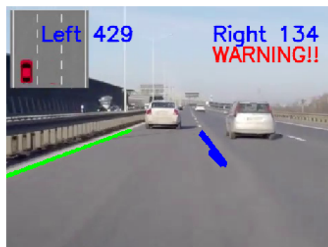
Figure 4.24. Example of lane assist, warning the driver that the vehicle has passed the crossing threshold.
