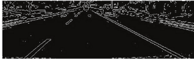
Figure 3.17. Edge detection based on Sobel operator. Taken from [65], © 2015 IEEE.
