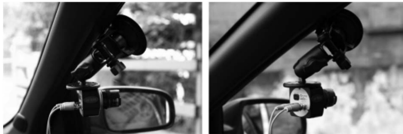
Figure 3.29. Camera is mounted on inside of right side window. Taken from [38], 2012 IEEE.
