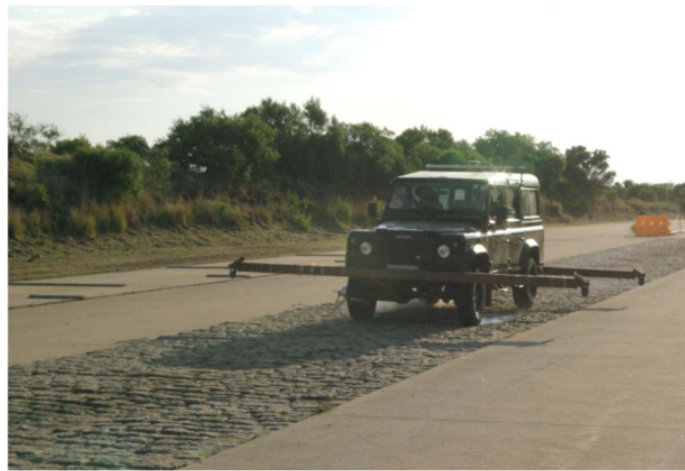
Figure 4.9: A test vehicle performing a brake test on Belgian Paving (Penny, 2016)
