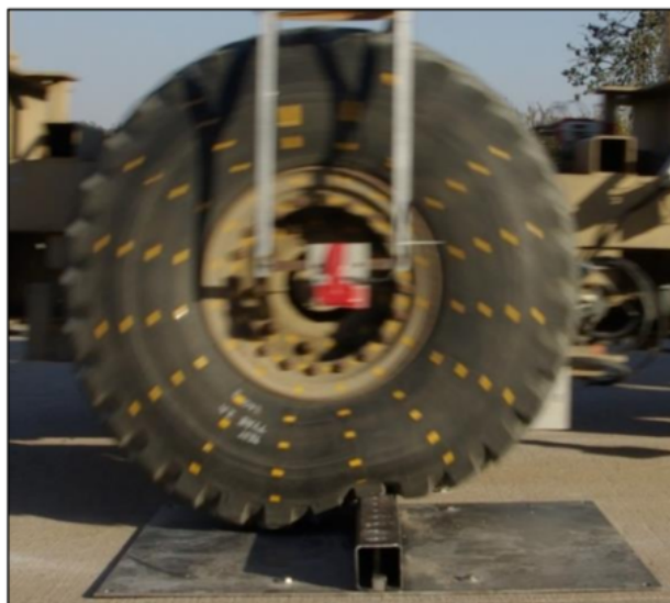
Figure 2.7: Tyre deformation as it rolls over a cleat (Hamersma, 2017)
