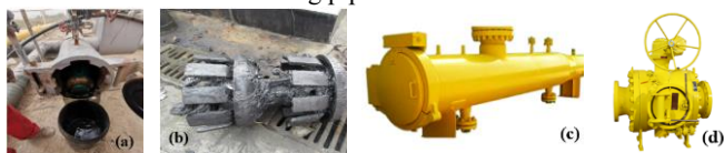
Fig.1 (a)Complex pipeline scene. (b)Oil and residues. (c)Non-standard transceiver device. (d)Pigging valve
