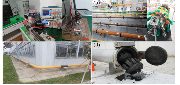
Fig.7 (a) Flat specimen detection. (b) Artificial pipe inspection. (c) Idle pipeline inspection. (d) Real pipe inspection.
