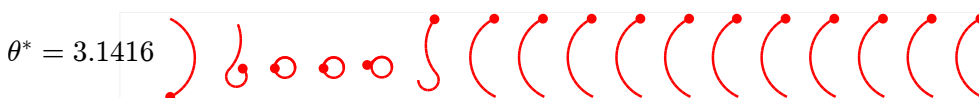
Figure 3.23: Turning gait prescribed by l_1 = 8.1, \kappa_1 = 2.25 . Visually, this shape aligns more closely with the Fourier k = 0.1 optimal turn for \theta^* = \pi , with initial and final posture, but is not the optimal in this shape space.
