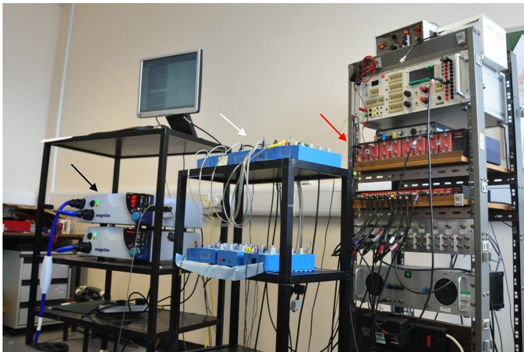
Figure 12: Equipment used in the experiments outlined in this thesis. Under the monitor is the Magstim 200 and Bistim (black arrow), with the ISO Dam amplifiers (white arrows) and CED data acquisition device (red arrow)
