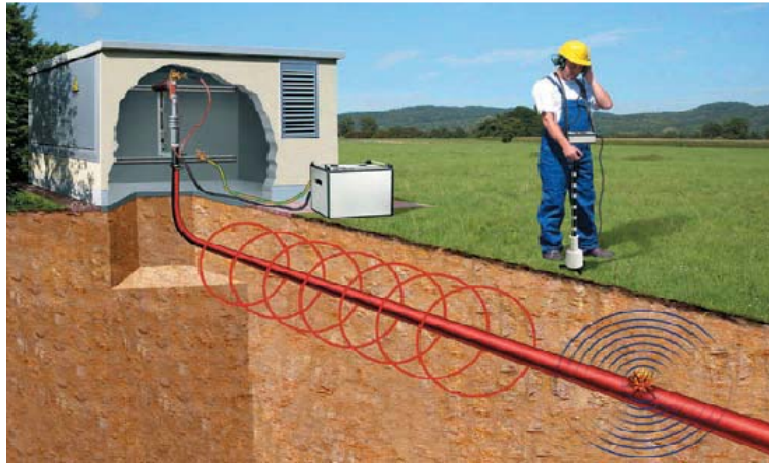
Figure 1.3: Thrumper method for underground short-circuit location.
