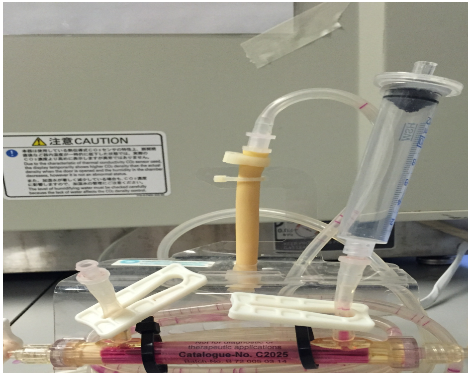
Figure 28 The modification of the bioreactor to permit transmural flow
