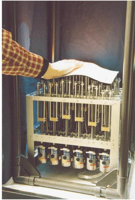
Figure 2.5-3. Project FEELEX haptic surface device. (Iwata, Yano, Nakaizumi, & Kawamura, 2001).
