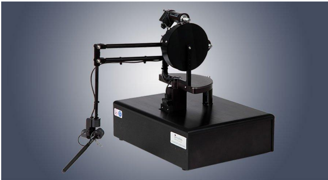
Figure 2.5-1. Phantom Premium 3.0 graspable kinaesthetic haptic device (Phantom 3D systems, www.3dsystems.com/haptics-devices/3d-systems-phantom-premium ).
