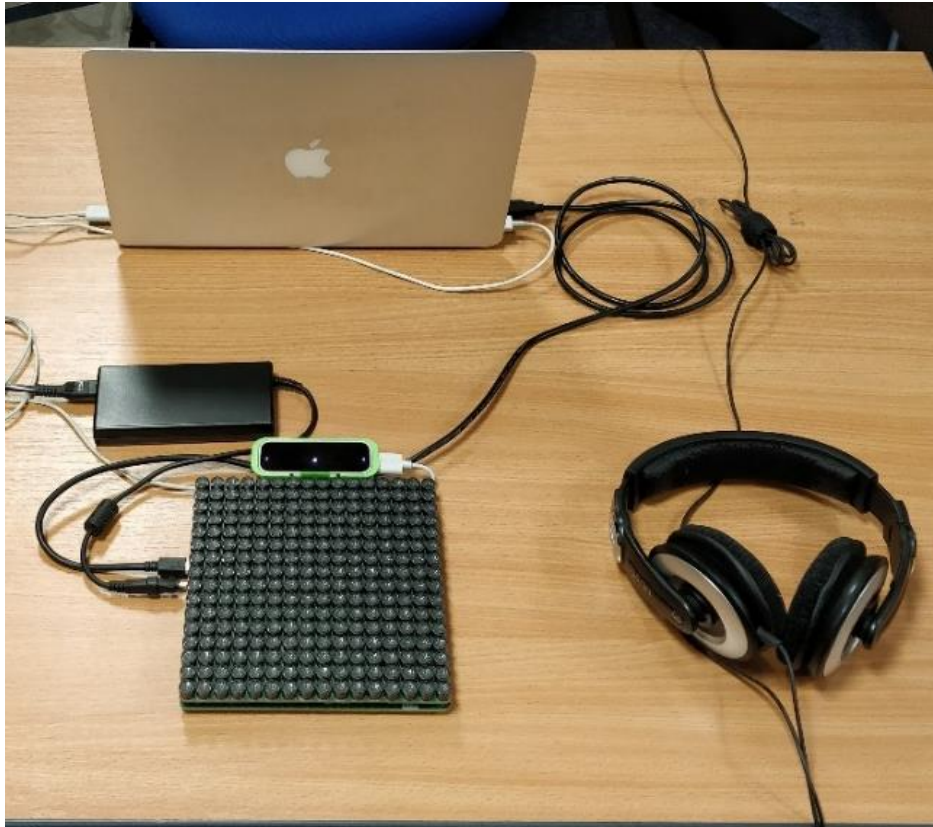
Figure 3.5-2. The UsHF equipment setup from the participant's location with the ultrasound array closest to them and the researcher's laptop opposite (left).
