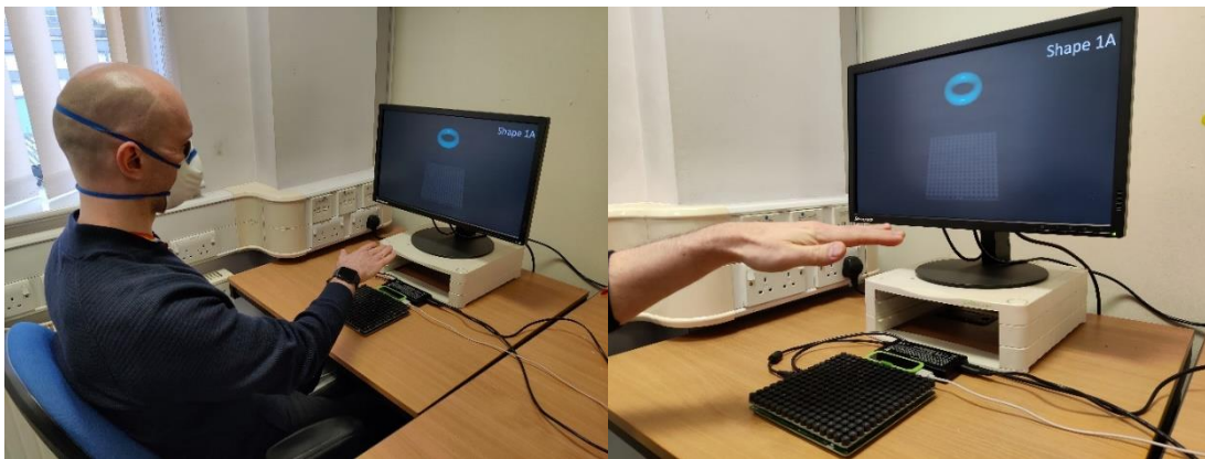
Figure 6.2-1. Two images of the current setup including the ultrasound array and monitor that was used to display visual stimuli during multimodal conditions.
