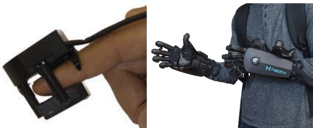
Figure 2.5-2. Fingertip haptic device (left) (Spagnoletti, et al. (2018) and HaptX DK2 haptic glove/hand exoskeleton (right) (HaptX, 2022).
