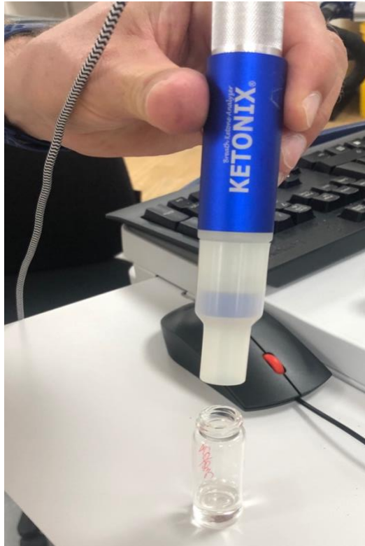
Figure 20: The Ketonix® placed over a container of liquid acetone to further ascertain the level of BrAce concentration variability the Ketonix® provides.
