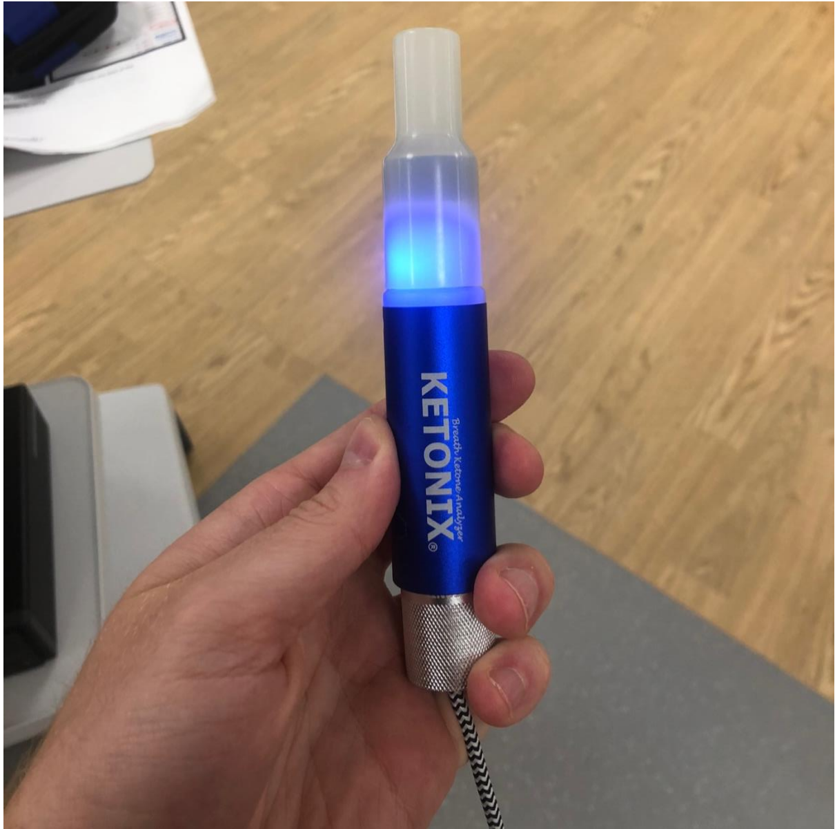
Figure 5: The Ketonix® with the accommodating mouthpiece attached.
