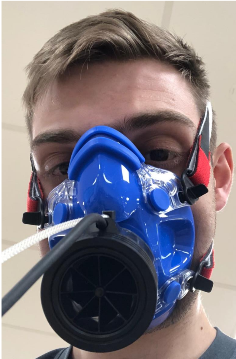
Figure 8: A pilot participant demonstrating how the turbine from the Cortex M3B connects to the Hans Rudolph V2 facemasks to collect gas analysis.
