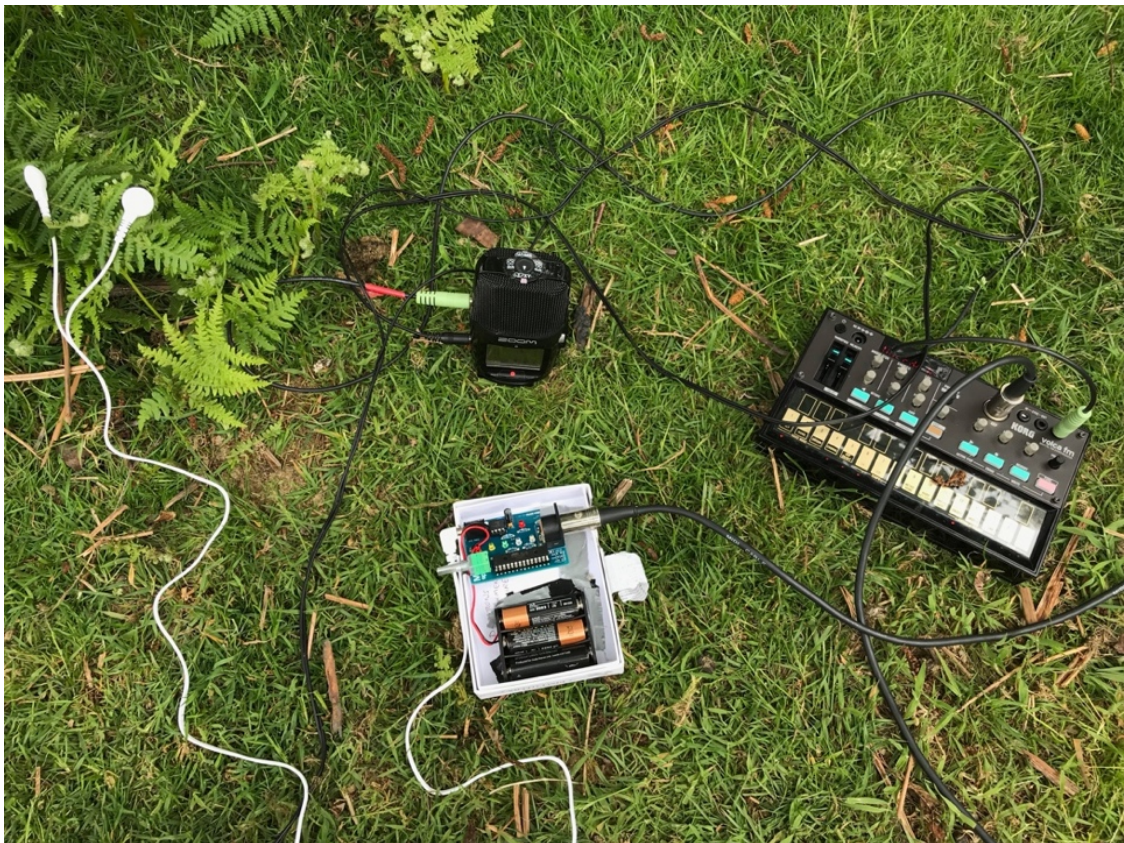
Fig 2. Biodata kit with electrodes, zoom HN2 microphone and Korg Synth sampling fern in Cardingmill Valley.
