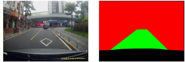
Segmentated Image (Green: Road, Red: non-Road Black: Removed Part)
