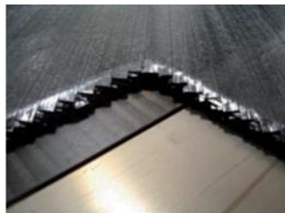
Figure 4: Ply edge with characteristic sawblade contour obtained by AFP process [coriolis composites, 2015]
