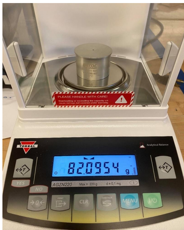
Figure 52: Total mass of barley grains measured using Torbal Analytical balance (Run#1)
