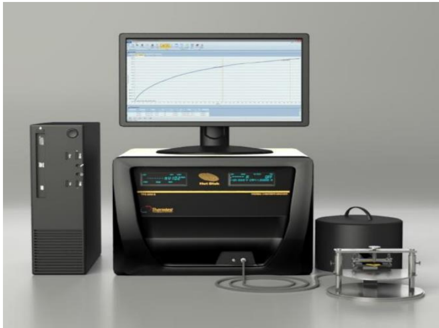
Figure 43: TPS 2500S Thermal Constants Analyzer [116].
