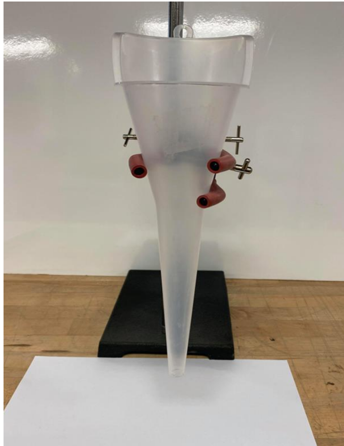
Figure 29: Flowability test set-up
