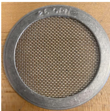
Figure 9: Sieve designation of 26 OPN (660.4 \mu\text{m} )
