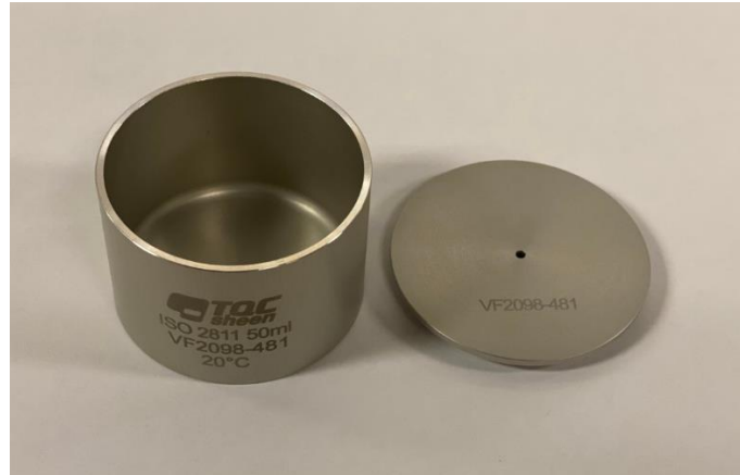
Figure 23: Aluminum Density Cup (pycnometer)
