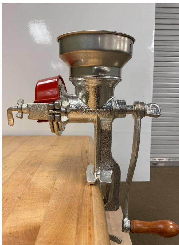
Figure 8: Manual low hopper grain grinder.
