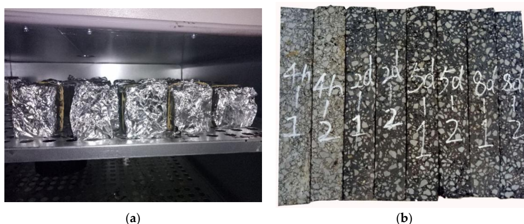
Figure 1. Specimen Aging (a) Set up in the Oven, and (b) Specimen after Oven Aging on Different Days.
