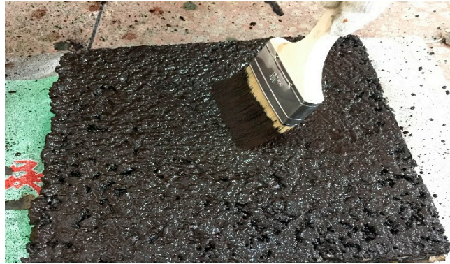
Figure 3. Painting the emulsified asphalt coating on the slab sample.
