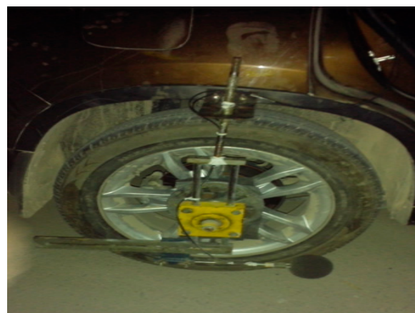
Figure 2. The on-board sound intensity system (OBSI).
