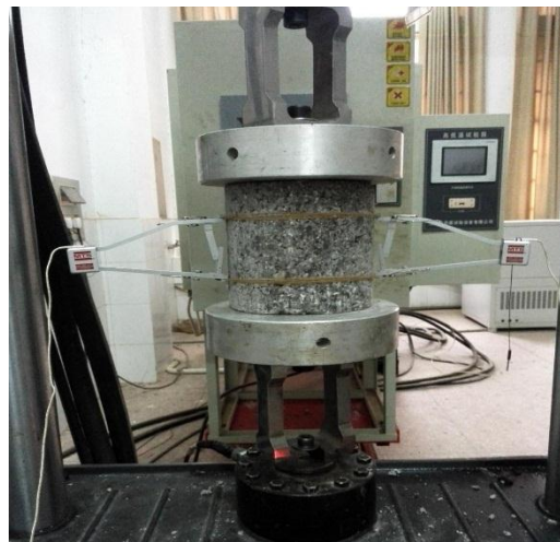
Figure 6. Device of compression resilience modulus test.
