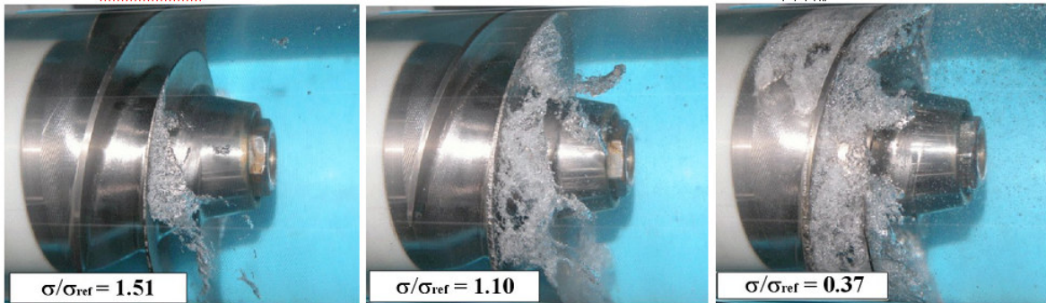
Figure 8. Cavitation inception and development on the FAST2 inducer for \phi/\phi_{ref} = 0.7 at room water temperature, \Omega = 3500 rpm and different values of the cavitation number.
