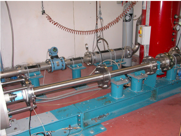
Figure 1. The Cavitating Pump Rotordynamic Test Facility.
