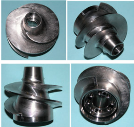
Figure 21. The FAST2 inducer.
