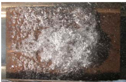
Figure 13. Cavitation appearance at higher freestream temperature ( \alpha = 8^\circ, \sigma = 2, T = 70^\circ C ).
