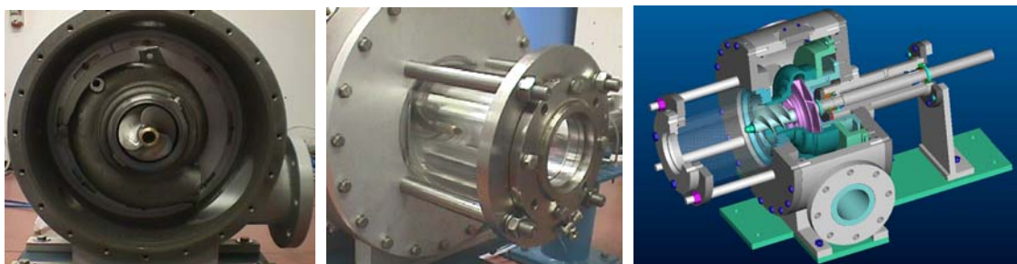
Figure 2 – The test section of the CPTF: the internal of the housing with the pump volute (left), the transparent inlet section (center), and a drawing of the test section assembly (right).
