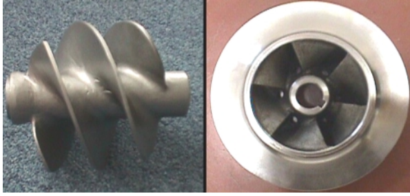
Figure 10. Axial inducer and impeller of the test pump used for CPTF validation.
