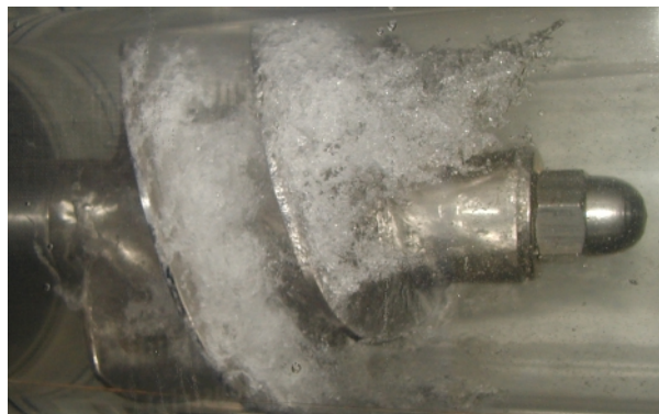
Figure 13. Extensive cavitation in the test inducer.
