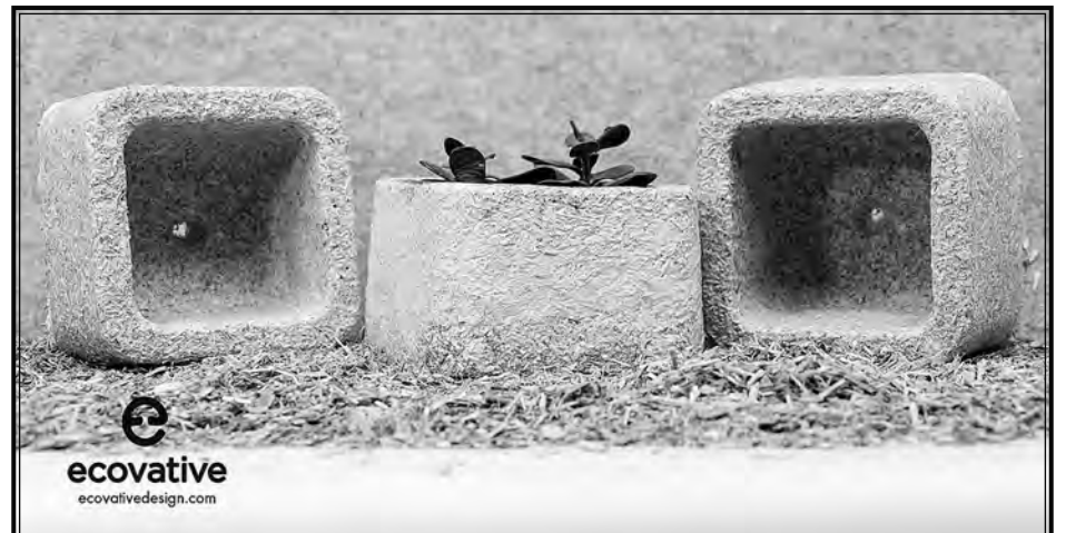
Buoyant, sturdy, mushroom material acts like plastic foam but will breakdown into compost. Photo courtesy of Evocative.
