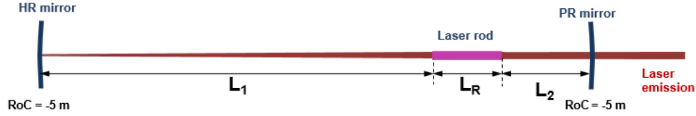
Figure 2.6 Schematic diagram of the TEM 00 -mode beam propagation along the symmetric laser resonator with large RoC (radius of curvature) mirrors.
