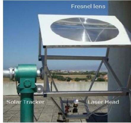
Figure 3.6 The Nd:YAG solar-pumped laser system with a 0.9 m diameter Fresnel lens and a laser head positioned in its focal zone.
