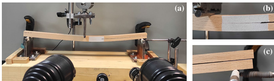
Fig. 6 a ENF specimen being tested; b detail of the fracture zone; c detail of the support
