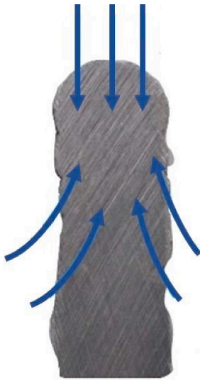
Fig. 8. Schematic representation of the cooling flow (arrows indicate the cooling direction).
