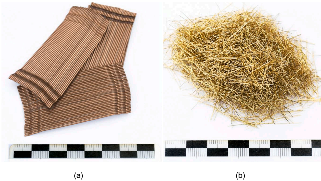
Fig. 1. Steel fibers used in HPFRC: a) Triple hooked-end hooked fibers with diameter 0.9 mm and length 60 mm; b) straight fibers with diameter 0.2 mm and length 13 mm (ruler divisions: cm and mm).
