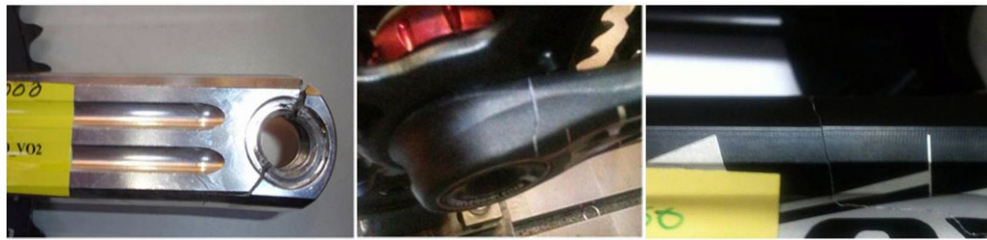
Figure 4 Appearance of cracks during fatigue tests.
