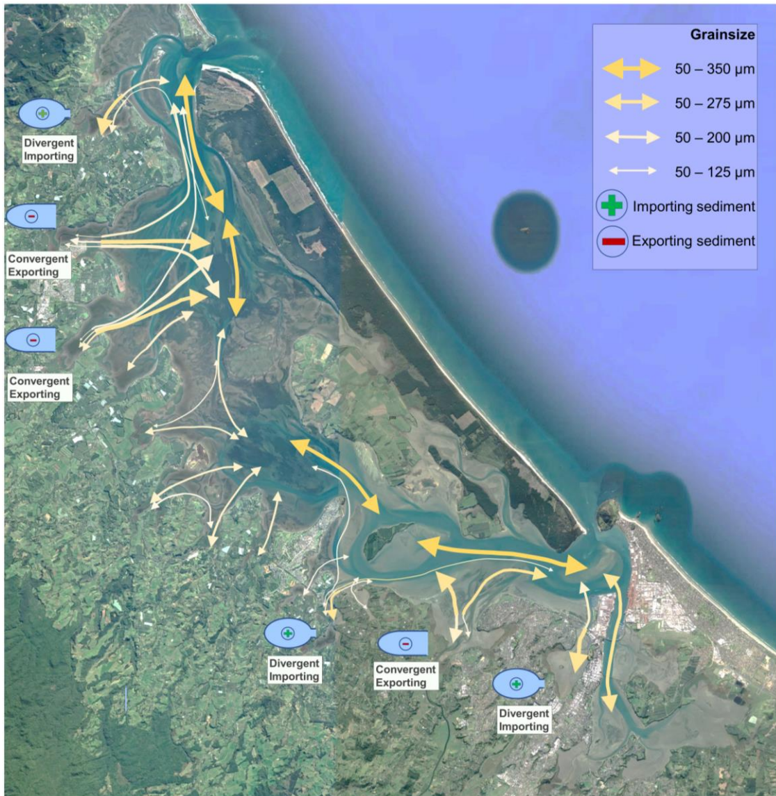
Figure 4.8: Conceptual model of the main sediment transport pathways in Tauranga Harbour, based on our sediment connectivity analysis. The arrows indicate the range of sediment grainsizes (colour) transported between the different estuary regions, and the relative strength of the connections (arrow size). Note that the different arrow ends may show transport of different sizes. The six divergent and convergent sub-basins are also highlighted in the figure (blue icons). Transport of coarse sediments ( >300 \mu\text{m} ) is mainly confined to the deep tidal channels, whereas sub-basins and upper estuary regions are characterised by transport of mainly finer sediment fractions ( <200 \mu\text{m} ).
