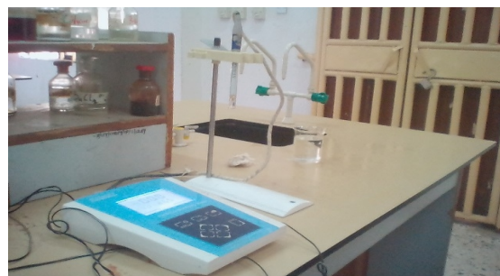
Figure 1: JENWAY 4510 conductivity metre
