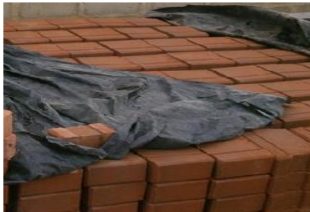
Figure 1. Stacked hydraform blocks Source: Nairaland Forum, 2020 [16].
