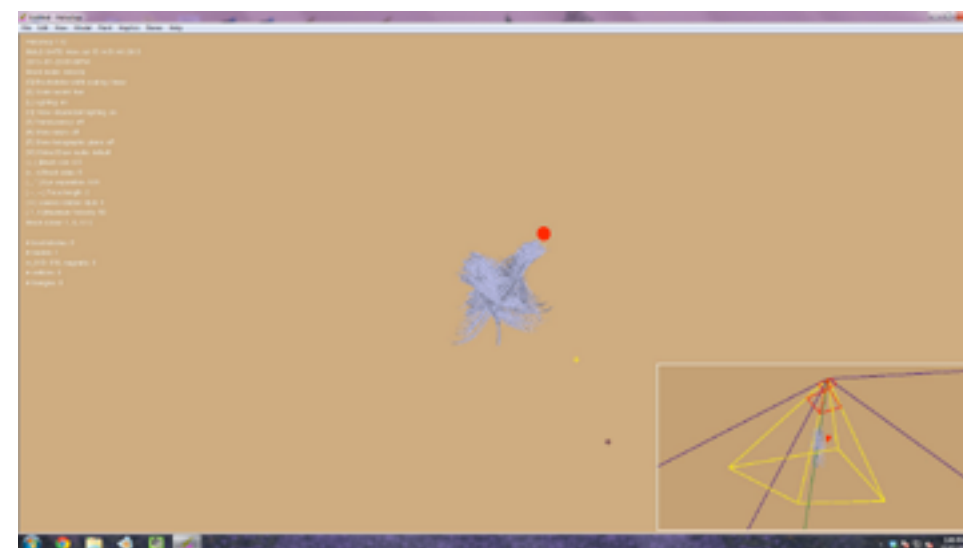
Fig. 19 - In the inset window the Haptic Frustum is shown in Yellow at a different size from View Frustum which is shown in Blue
