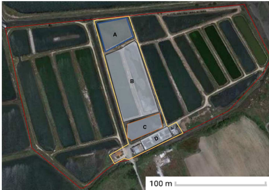
Figure 14. Company area (in red), including the production area (in yellow), where Water capture (A), Fish production (B), Sedimentation tank (C) and Seaweed production (D) are inserted. (Google Earth, 2021 (adapted))
