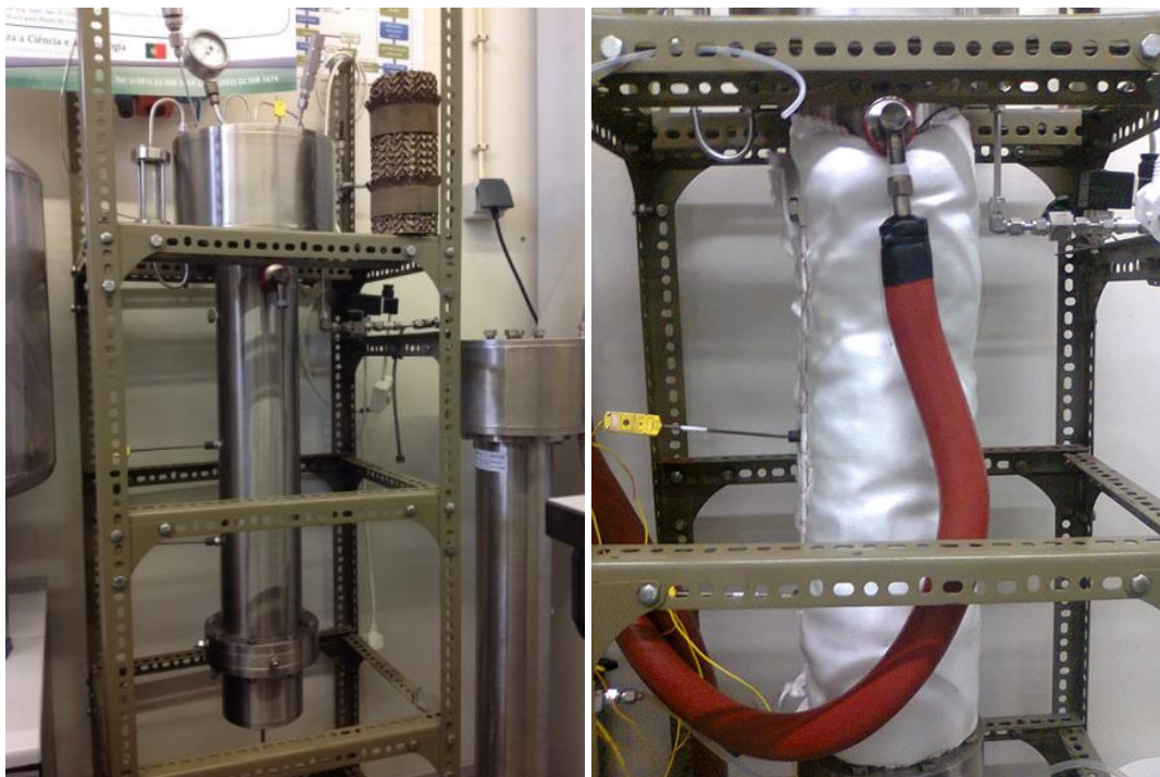
Figure S 1 – Picture of the structured packed bubble column reactor, a Mellapak Y50 packing element is visible (left) and with the heating oil tubes and thermal insulation jacket mounted and the middle thermocouple is also visible.
