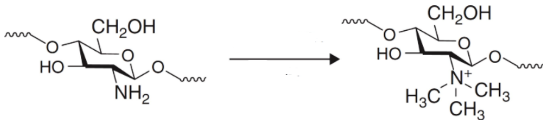
Figure 1. 6- Quaternization reaction of chitosan amino groups, giving rise to N, N, N-trimethyl chitosan. Adapted 117
