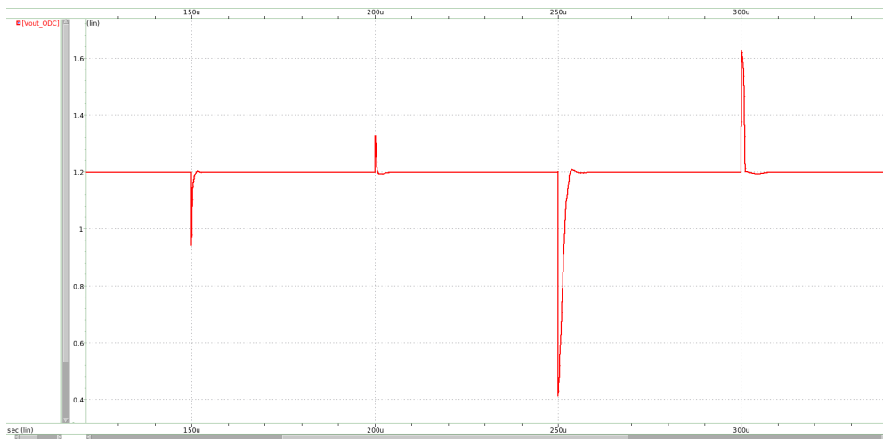
Figure 4.5: Load transient simulation of the ODC
