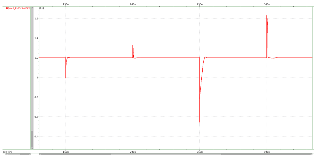
Figure 4.7: Load transient simulation of the Full Spike Detection Circuit
