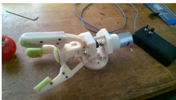
Fig.5. Prototype gripper built using 3D printing
