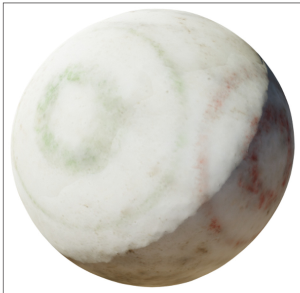
Figure 6 Photogrammetric model of marble. Model created in Agisoft Metashape, image rendered with artificial lighting in Blender.
