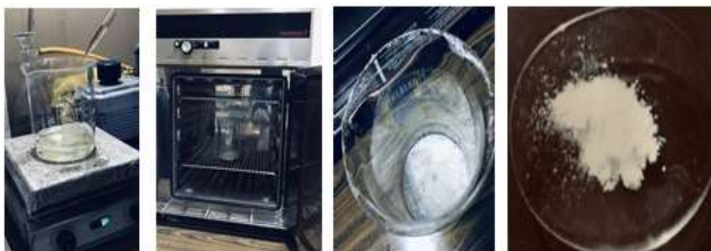
Figure 2: Steps of synthesis MgO using Sol-gel technique
