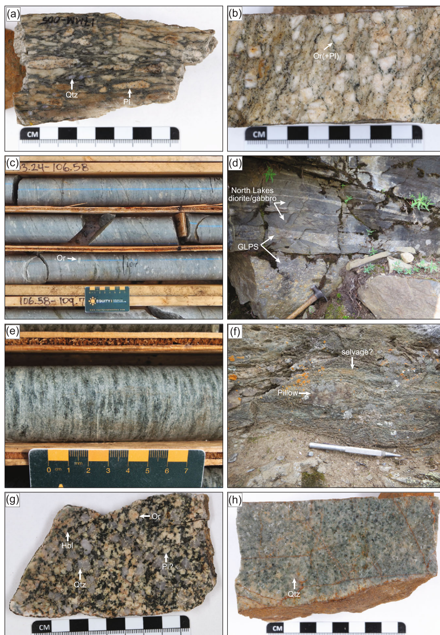
FIGURE 7: Photographs of representative felsic and mafic volcanic, high-level intrusive, and plutonic rocks in the Big Campbell (a–f) and Cleaver Lake (g, h) thrust sheets, Finlayson Lake district. (a) 17MM-005: Grass Lakes plutonic suite: foliated and deformed, massive plagioclase feldspar-quartz granodiorite; (b) 18MM-105: massive, equigranular, moderately foliated granodiorite; (c) 17MM-061: Grass Lakes plutonic suite, high-level quartz-orthoclase feldspar porphyritic rock with rare blue quartz eyes that cuts Kudz Ze Kayah deposit footwall; (d) 18MC015/96DM-065: North Lakes intrusion, fine to medium-grained gabbro to diorite intruded by Grass Lakes plutonic suite granitic dikes; (e) 18MM-132: Kudz Ze Kayah formation (Krakatoa zone), high-level chlorite-altered mafic dike in the Krakatoa deposit footwall; (f) 17MM-054: Wind Lake formation, deformed and altered pillow basalts with possible outer selvage; (g) P99-24: Simpson Range plutonic suite, equigranular hornblende granodiorite; (h) 18MM-108: Cleaver Lake formation, high-level quartz-porphyritic intrusive rock. Hammer (35 cm) for scale in (d) and pen (10 cm) for scale in (f). Qtz = quartz; Or = orthoclase; Pl = plagioclase; Hbl = hornblende.
