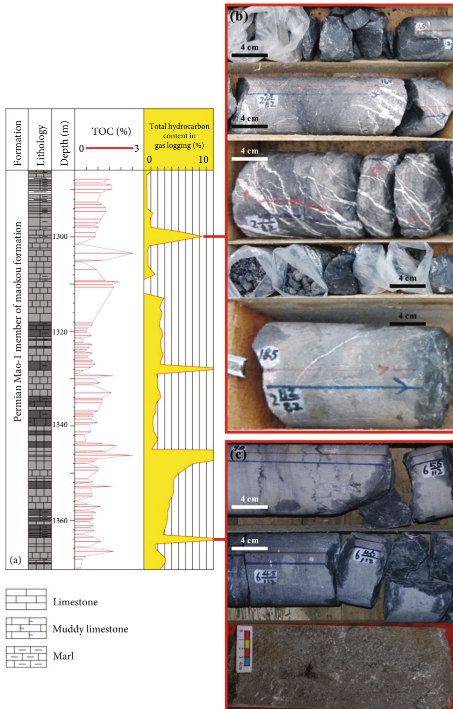
FIGURE 9: (a) Correlation profile between gas logging total hydrocarbon contents and TOC values for Permian Mao-1 member of Maokou Formation in JY66-1. Development of fractures at the peak of gas logging in JY66-1: (b) 1297-1302 m and (c) 1363-1365 m. JY = Jiaoye.
