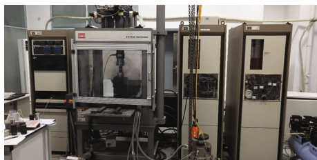
FIGURE 4: MTS816 electrohydraulic servo rock test system.
