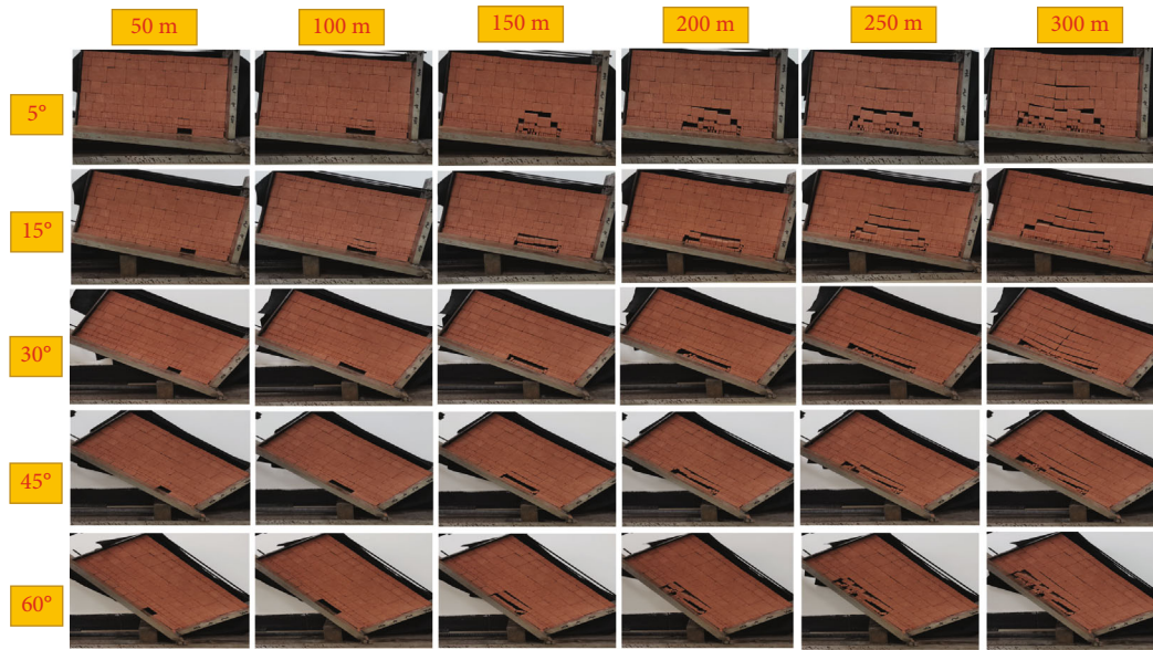
FIGURE 6: Collapse characteristics of disturbed overburdens during simulated mining of inclined coal seams at different dip angles and different excavation lengths.
