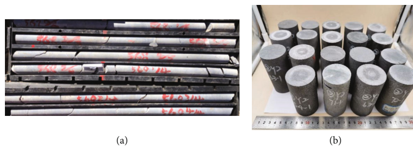
FIGURE 2: Sandstone cores and sample specimens. (a) Core obtained from field drilling. (b) Standard specimens made from rock cores.
