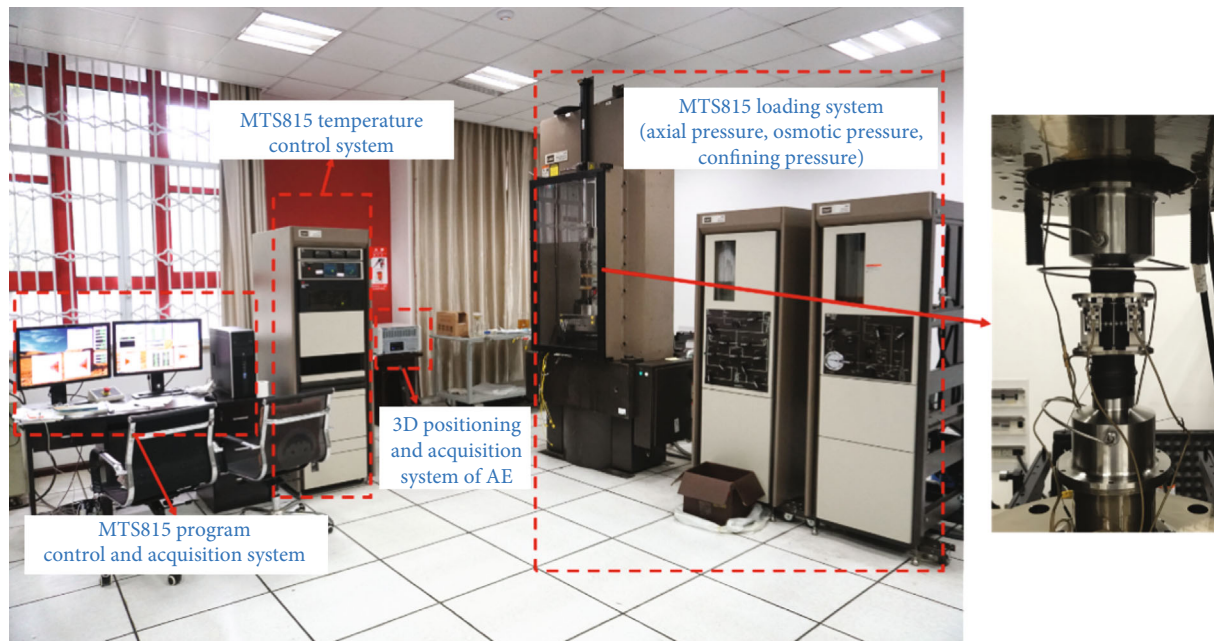
FIGURE 3: MTS 815 Flex test GT test system.
