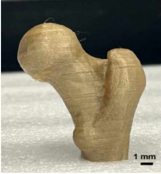
Figure 1.10: Photograph of a femoral head as developed by the optimized set of printing parameters (Nozzle temp: 4100C, Chamber temp.: 900C, Printing speed: 50 mm/sec, Layer height: 0.1 mm) and LD filaments.
