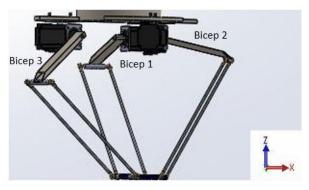
Fig. 8. Labelled bicep of a delta robot arm.
