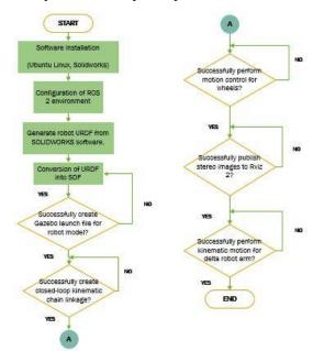
Fig. 1. The flow chart of the simulation development
