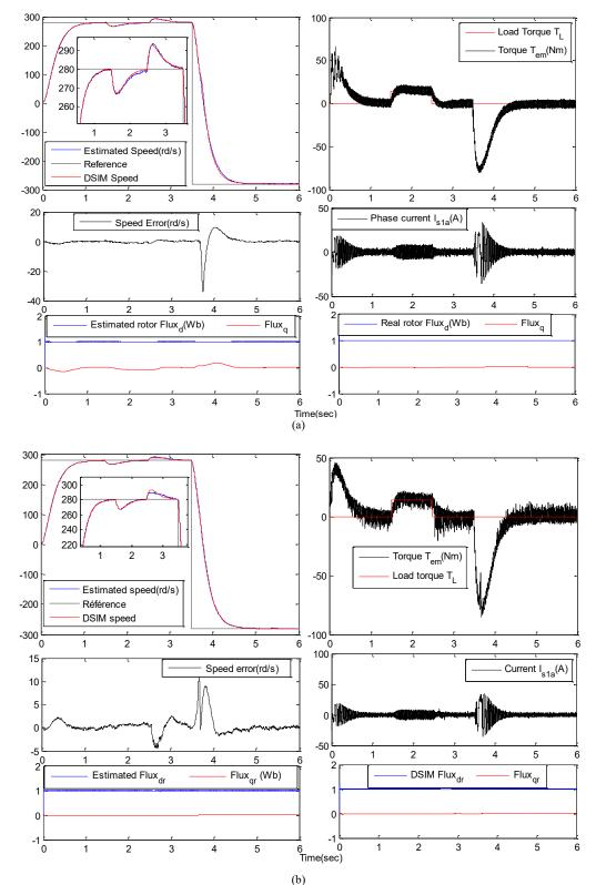
Fig. 3. Simulation results for sensorless direct vector control of DSIM. (a) proposed state observer. (b) SM-MRAS estimator [32].
