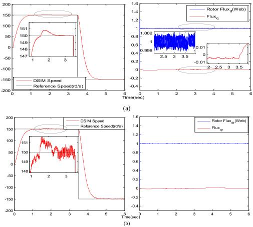
Fig. 6. Parameter variation of +50% R<sub>s1,2</sub>; for nominal speed test. (a) proposed state observer. (b) SM-MRAS estimator [32].
