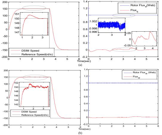
Fig. 8. Parameter variation of -50% Lm; for nominal speed test (a) proposed state observer (b) SM-MRAS estimator [32].
