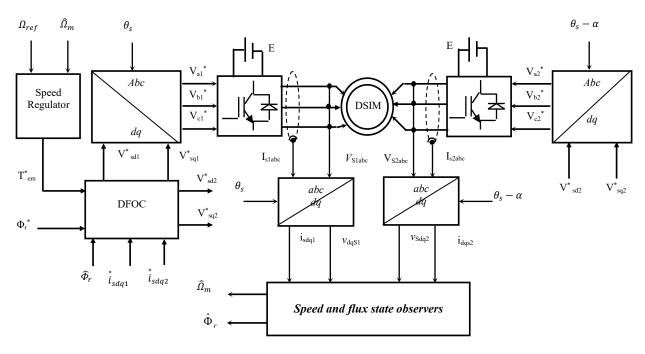
Fig. 1. Sensorless vector control scheme of DSIM
