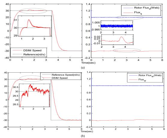
Fig. 11. Parameter variation of +100% J; for a low-speed test (a) proposed state observer (b) SM-MRAS estimator [32].
