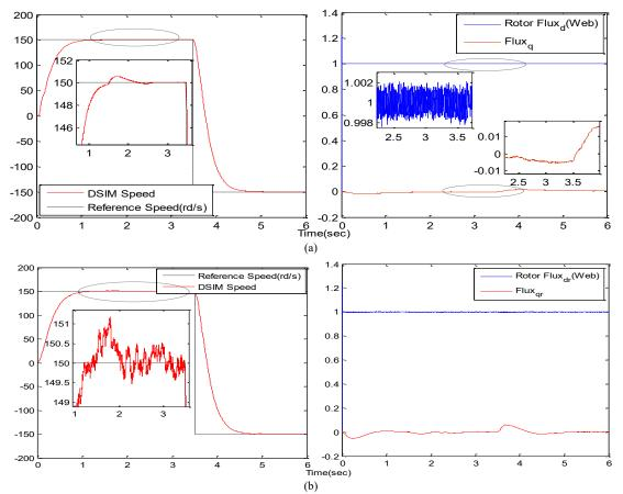
Fig. 10. Parameter variation of +100% J; for nominal speed test (a) proposed state observer (b) SM-MRAS estimator [32].
