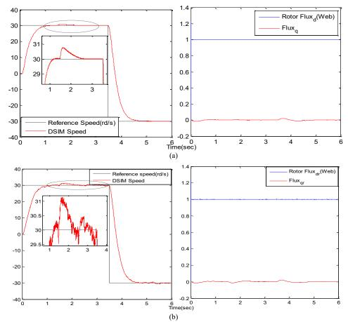
Fig. 5. Parameter variation of +50%Rr; for a low-speed test (a) proposed state observer (b) SM-MRAS estimator [32].
