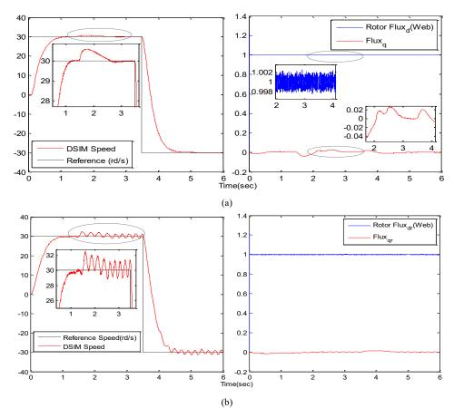
Fig. 7. Parameter variation of  $+50\% R_{s1,2}$ ; for low-speed test. (a) proposed state observer. (b) SM-MRAS estimator [32].
