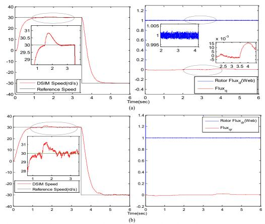
Fig. 9. Parameter variation of -50% Lm; for a low-speed test (a) proposed state observer (b) SM-MRAS estimator [32].
