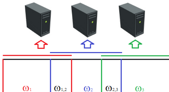
Fig. 8.1: Partition of the domain \Omega into three overlapping subdomains \omega_1, \omega_2 and \omega_3 with overlaps \omega_{1,2} and \omega_{2,3} .
