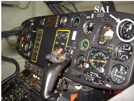
Figure 10. The developed SAI attached on the helicopter simulator panel.
