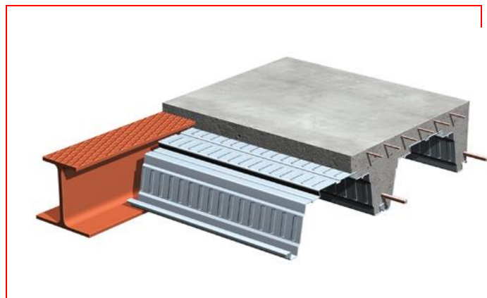
Fig. 1 Typical asymmetric slim floor beam layout
