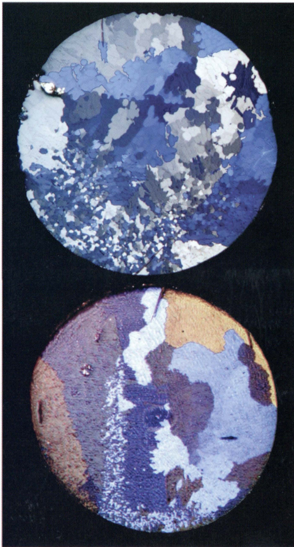
The growth of tin crystals from a tin melt containing a dash of silver changes dramatically as a third element, copper, is added.
