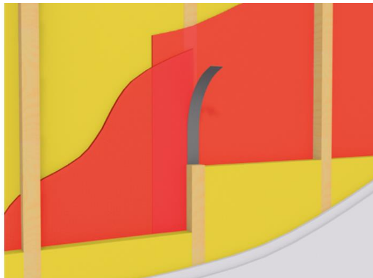
Figure 1 Exterior timber stud wall, where the vapor barrier (shown in red) is mounted on the warm side of the thermally insulated exterior building envelope. The webs of the membrane must overlap on a solid surface and be joined together with adhesive or tape (shown in grey)
